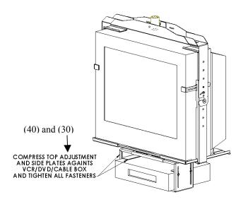
Figure 8. Make Adjustments to Unit
